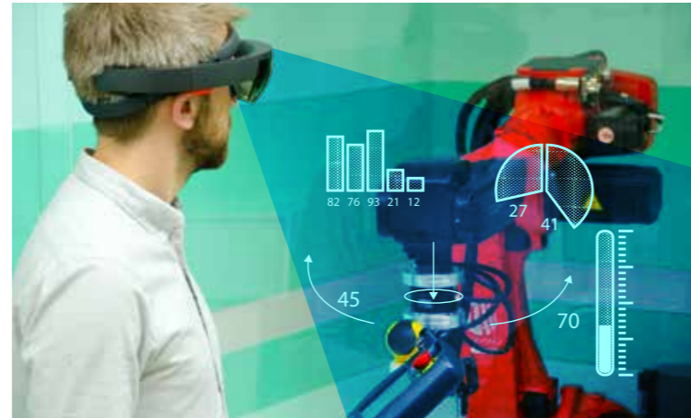
The interplay between modular shop floor IT and the machine twin enables context-sensitive delivery of current relevant machine and process data to workers.
