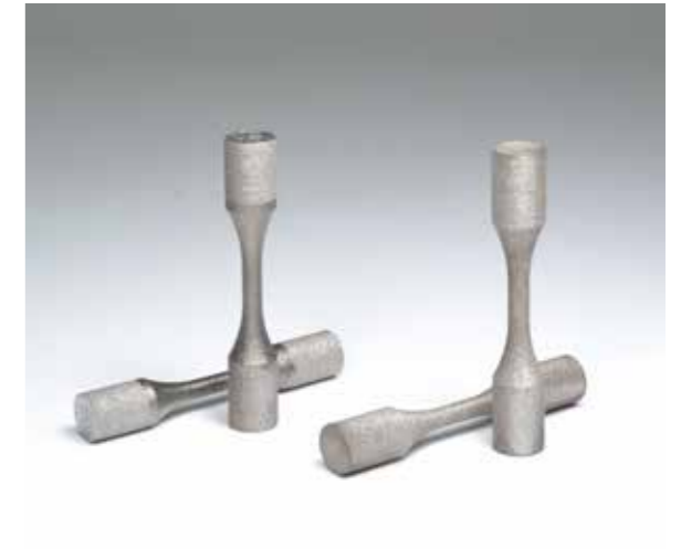
Generated test specimens for mechanical characterization of titanium alloy parts produced by SLM
