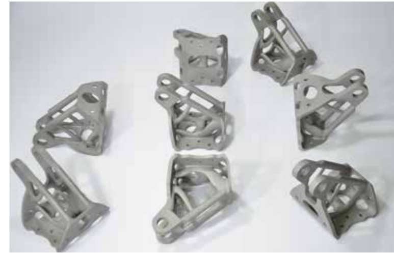
SLM-structural prototypes for airplanes produced at Fraunhofer IPK for Embraer
